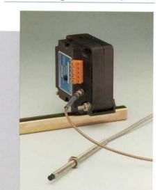
This proximity type vibration sensor is the most widely used sensor to measure vibration and position movement of machine elements. This noncontacting sensor provides highly accurate measurement of vibration amplitude, eccentricity, static shaft position or dynamic motion. The sensor operates on the Eddy current principle.
